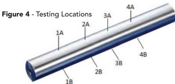
The testing program first considered magnetic pull force. To perform the test, a ¼ inch steel ball was placed on the magnetic pole locations and pulled perpendicular to the surface of the tube magnet.
