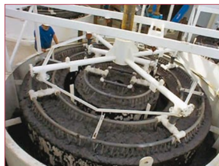
Figure 12. 4.6 m (15 ft) diameter CoalPro column flotation cell with an adjustable wash water system. The wash water removes entrained clays from the coal froth.
