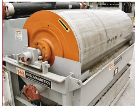
Figure 6. Wet drum magnetic separators for heavy media application. Self-levelling counter-rotation tank style.
