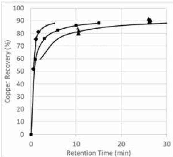
Figure 4: Kinetic recovery curves for the StackCell train (diamonds), Denver batch test (squares) and industrial tank cells (triangles)
