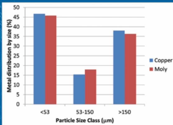
Figure 1: Metal contained in the final tailing stream of a large copper concentrator
