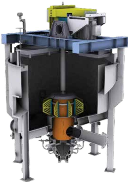
**Figure 2: Cutaway of the Eriez StackCell™ illustrating the concept of the tank within a tank**
