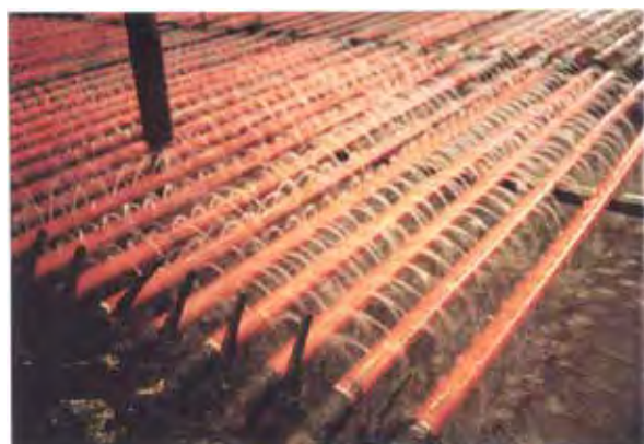
FIGURE 2 The use of wash water improves concentrate quality
