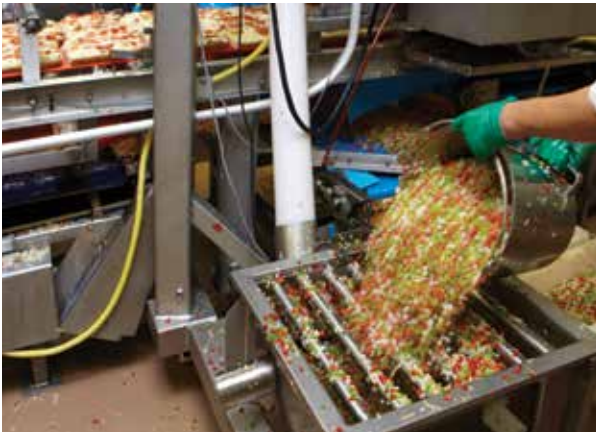
Magnetic grates allow free flowing product to pass between the magnetic tubes.
