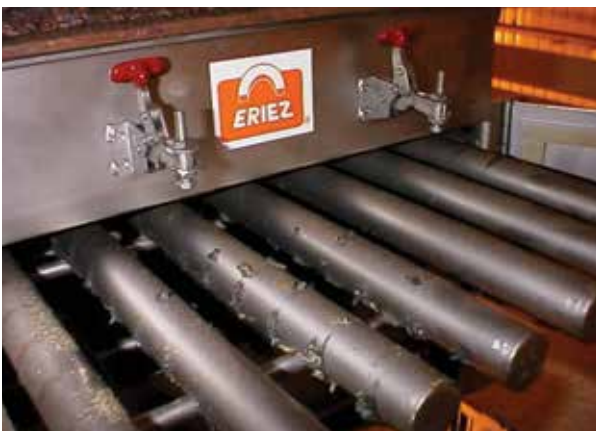
Iron particles are held against the magnetic tubes.
