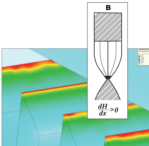
Schematic 1: The DVMF's matrix converges the lines of magnetic flux for improved collection of magnetic contaminants.
