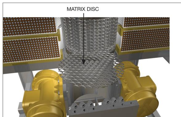
**Figures 2 and 3: The DVMF consists of a thick steel box with a canister in the bore. Aluminum or copper coils are positioned around the canister. Direct current power energizes the coil and allows the matrix to collect magnetic particles.**
