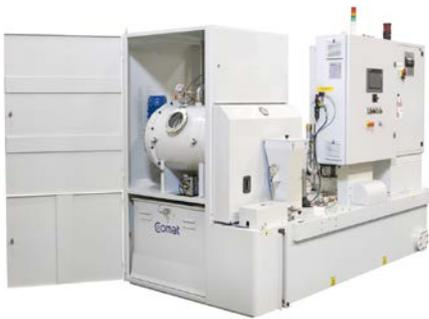
Erie, PA—In 2016, [Eriez® HydroFlow®](#) partnered with Milan, Italy-based [Comat S.r.l](#) to bring [SuperFiltration technology](#) to North America, providing customers a long-awaited solution to remove particles down to 3-micron nominal from cutting fluid while maintaining a stable fluid temperature. Eriez reports this breakthrough technology is generating strong activity and a positive response from the marketplace.
