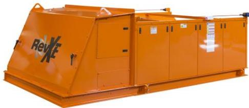
Erie, PA—Successful installations prove that Eriez® Ultra High-Frequency (UHF) Eddy Current Separators (ECS) successfully recover micro-fine aluminum, copper and other nonferrous fines from automobile shredder residue (ASR) that is missed by traditional machines. “Field results demonstrate this separator’s ability to reliably recover fine nonferrous metals, including bare copper wire, as small as 2-3 millimeters in size,” says Eriez Separation Product Manager Chris Ramsdell.
