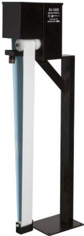
The Oil Skimmer squeezes oil between rollers, a method of stripping the oil from the belt that does not require scraping. This skimmer is designed for use on large machine tools with tanks deeper than two feet. The Oil Skimmer Jr. is designed for machine tools with shallow tanks.
