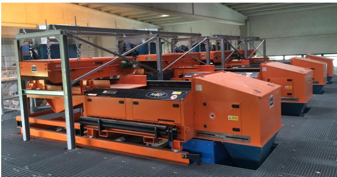
For complete metal recovery, Eriez manufacture a range of modular systems to separate ferrous and non-ferrous metals, designed to incorporate additional separators including overband magnets and magnetic drums, into stand-alone systems.
