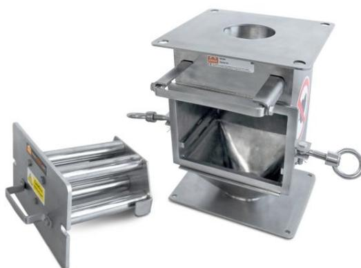
The permanent magnetic separators have been successfully installed throughout companies in the UK, removing fine and weakly magnetic particles from material flow. They are available in 152mm (6") and 203mm (8"), with a stainless steel housing, slide gate to shut off material flow, two banks of Rare Earth permanent magnets to 120°C and suitable for use up to 120°C.
