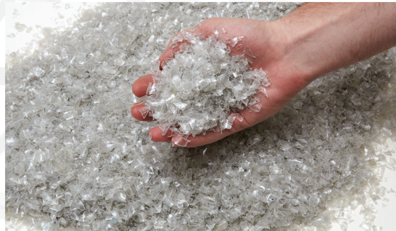
PET Flake is processed to remove tiny aluminum contaminants.
