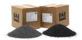
Ordinary plastics cannot be detected by metal detectors or x-ray machines. However, by incorporating new additives during manufacturing, broken pieces or fragments of plastic materials can be detected by a metal detector before getting mixed in with food products. This allows manufacturers to prevent contaminated products from reaching the market. Detectable additives can be infused during manufacturing to slightly magnetize some
