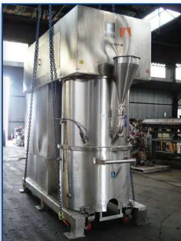
150 Gal. Ross Double Planetary Mixer, Model DPM 150, 316L S/S, Unused - Item: 36540
