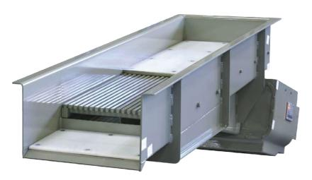
The units function as surge pile discharge feeders and meter minus 2 \( \frac{3}{4} - in. \) stone to an inline belt conveyor.
