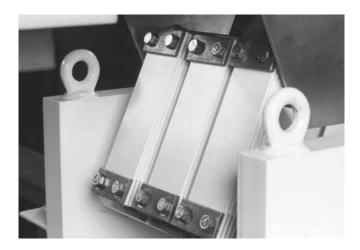
The VMC Conveyor is designed to be maintenance free and no periodic maintenance is required. If the leaf springs become damaged by accident or abuse, they must be replaced.
