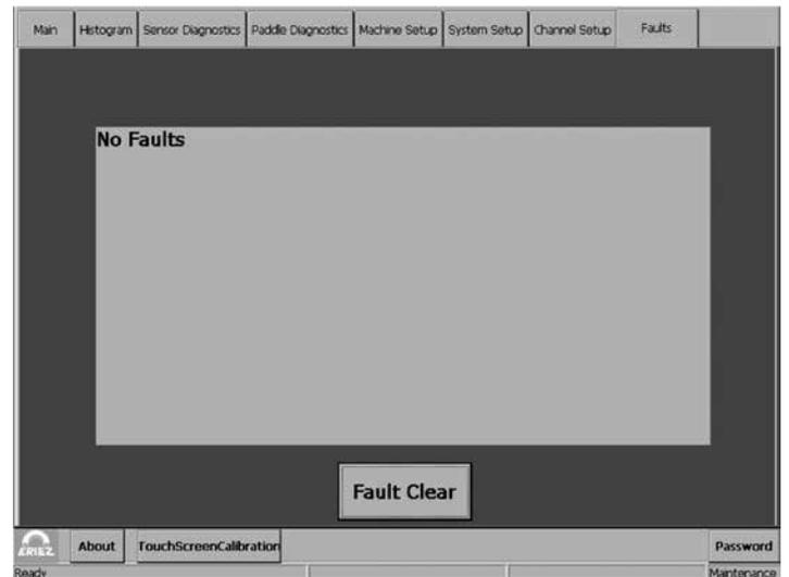
The “Faults” Screen will show details about any faults that are occurring in the system. This screen is the first place to check if the system is not functioning properly.
