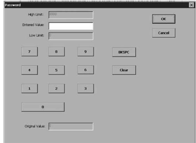
The “Numeric Keypad” is used whenever a numerical value needs to be entered. The name of the parameter that is being changed is shown in the title portion of the keypad. In this example, the ‘Password’ is being entered.
