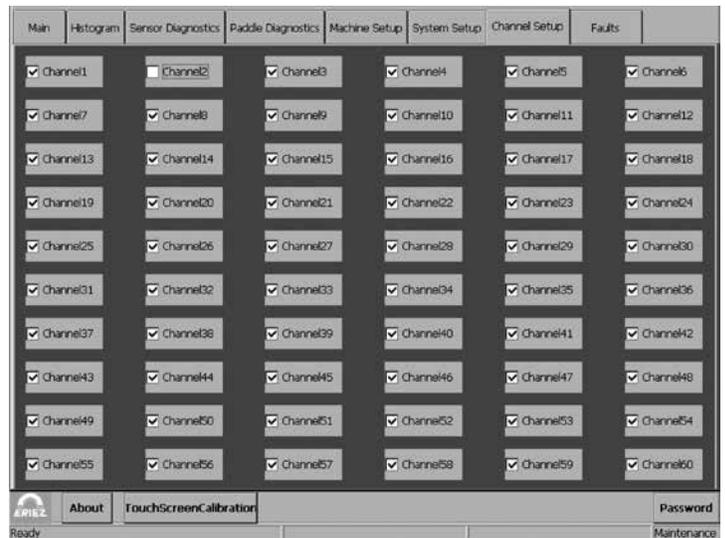
The "Channel Setup" screen can be used to enable/disable a single channel in the system for troubleshooting or if a failure occurs. A channel is made up of a sensor, electronics, and a paddle. Disabling the channel will notify the software to stop monitoring the sensor and to remove power from the corresponding paddle.
