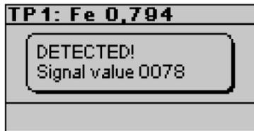
If the signal exceeds the configured value, the user can only reject the result.
