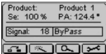
Should an error occur, the following mask is displayed, the red error light flashes and a log entry is created. The picture shows a light barrier error as an example. The error message can be reset by pressing the RESET button, once the cause of the error is corrected.
