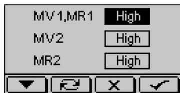
Select output with F1 . Change between "Low", "High" and "Inactive" with F2 . Exit menu without any changes with F3 . Confirm changes and exit menu with F4 .
