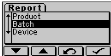
**PLEASE NOTE:** The report is output through the serial COM2 interface in formatted form. A maximum of 42 characters is output per line. Each line ends with LF (linefeed, ASCII 0Ah). Every report can be directly printed with the EM report printer (option).
