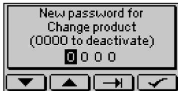
A password assigned previously has to be entered before a new one can be assigned.
