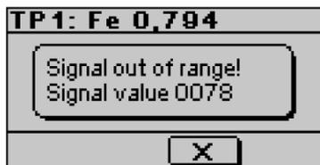
Steps 2 and 3 are now repeated for all defined tests samples. The error message on the left will appear, should one of the tests be unsuccessful or was not started on time and the device has been configured accordingly. The red fault LED will flash. The output "LF" will be deactivated.
