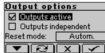
**Outputs active:** Inactive outputs are not activated upon metal detection; no log entry is created. The operating mask displays "Output OFF".
