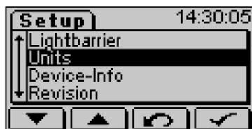
Country specific conveyor speed display and time and date formats can be configured here. Formats for conveyor speed:
