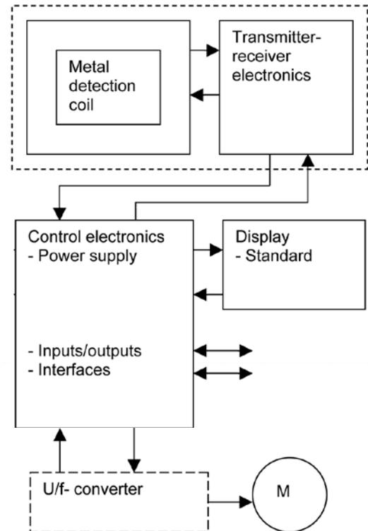
The metal detector works with the so-called “balanced coil” principle:
