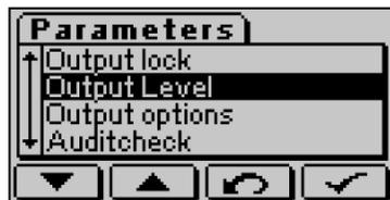
Select output with F1 . Change between "Low", "High" and "Inactive" with F2 . Exit menu without any changes with F3 . Confirm changes and exit menu with F4 . If the outputs are **not** marked as independent (See Change Password – Outputs (Options)), MV1/2 and MR1/2 are setup together.
