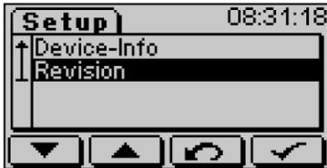
Version number of the installed hardware and software components of STE and AWE are displayed. Exit menu with F4 .
