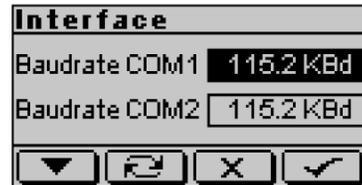
Select device address with F1 /F2 . Exit without changes with F3 . Confirm with F4 .
