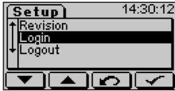
Enter login code with F1 , F2  and F3  and confirm with F4. To exit the menu, sign out (see Menu/Operation - Logout) or restart the device.
