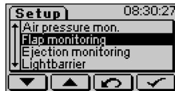
Flap monitoring can be configured in this menu. 0.0s deactivates the monitoring. Values different than 0 set the time, which the flap may not extend when switching from normal position to reject position and vice versa. The value can be varied in steps of 0.2s up to a maximum of 20.0s. Changing the factory pre-set value is usually not required.
