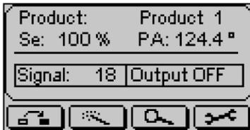
If metal detection is deactivated over the digital bypass, the display shows **ByPass**. In addition, the green operating light is off as well and a log entry is created.
