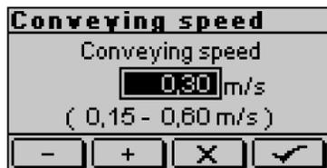
Depending on selected velocity unit, values are displayed in m/s, m/min, ft/s or ft/min.
