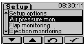
The air pressure can be monitored. 0.0s deactivates the monitoring. A value different to 0 sets the maximum time, in which the air pressure can drop below the limit set in the pressure controller without creating an error message. The value can be varied in steps of 0.5s up to a maximum of 5.0s. Changing the factory pre-set value is usually not required.
