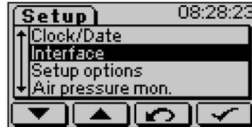
Select interface COM2 (plug 7b) or COM1 (plug 11) with F1 . Select baud rate with F2 . Confirm with F4 or exit without changes with F3 .
