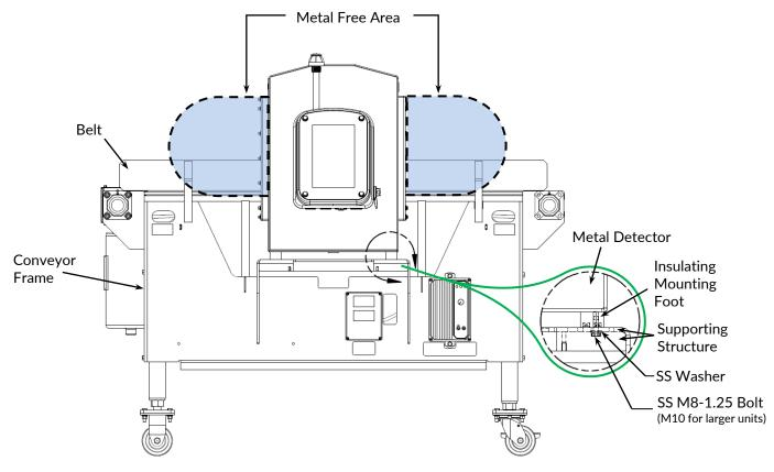
Figure 9: Metal free area and mounting feet
