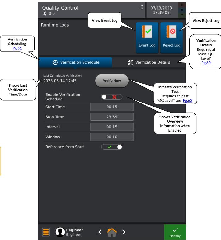
NOTE: The verification window opens the set number of minutes prior to the next verification check and closes at the time when the verification check is overdue. A warning will be displayed when the window opens and a fault when it closes if the verification check was not completed.
