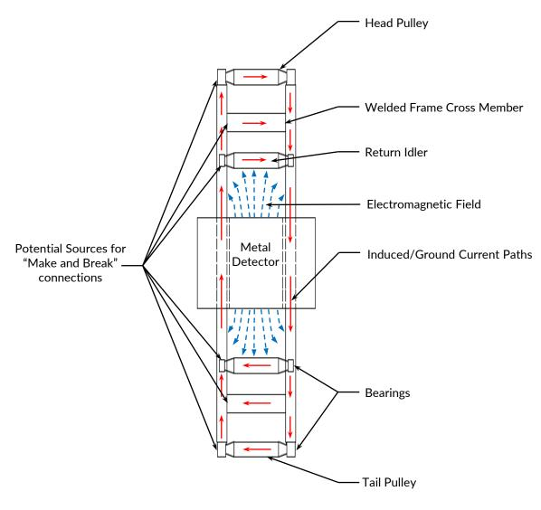
Figure 4: Potential sources for "Make and Break" connections
