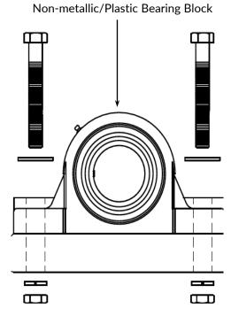
Figure 7: Recommended method for insulating bearing block
