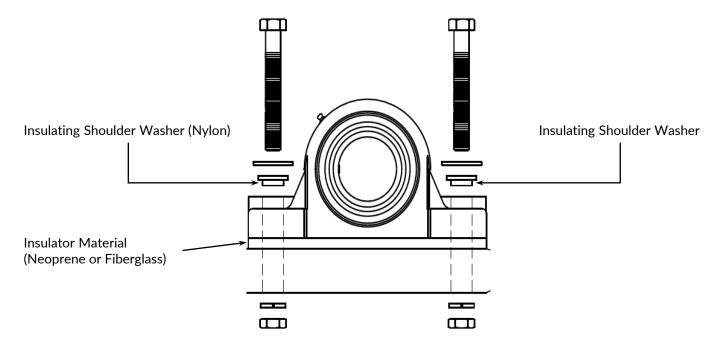
Figure 6: Bearing block on conveyor frame
