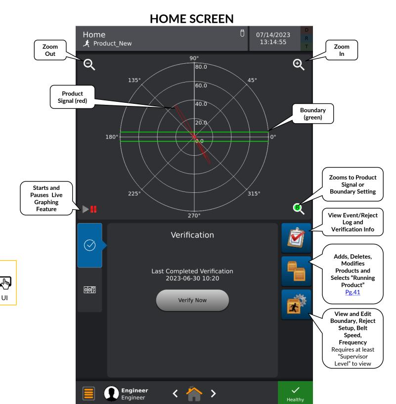
NOTE: This is the default screen when the detector is initially turned on.
