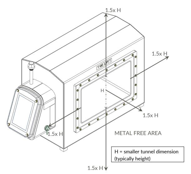
Figure 3: Metal free area for a tunnel type metal detector
