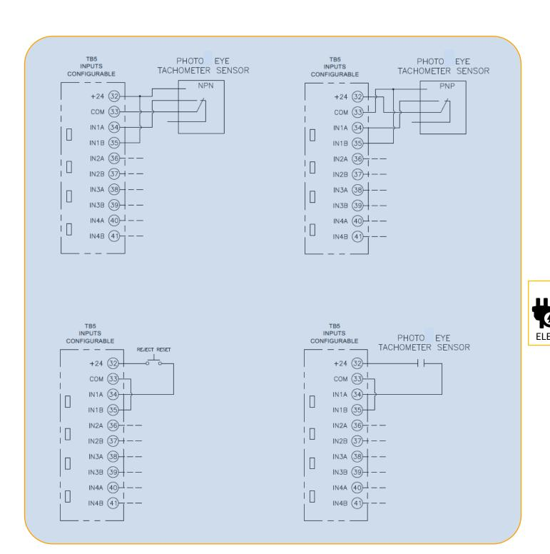
Figure 15: Input connection examples
