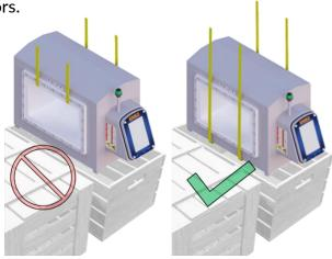
Figure 1: Metal detector handling instructions
