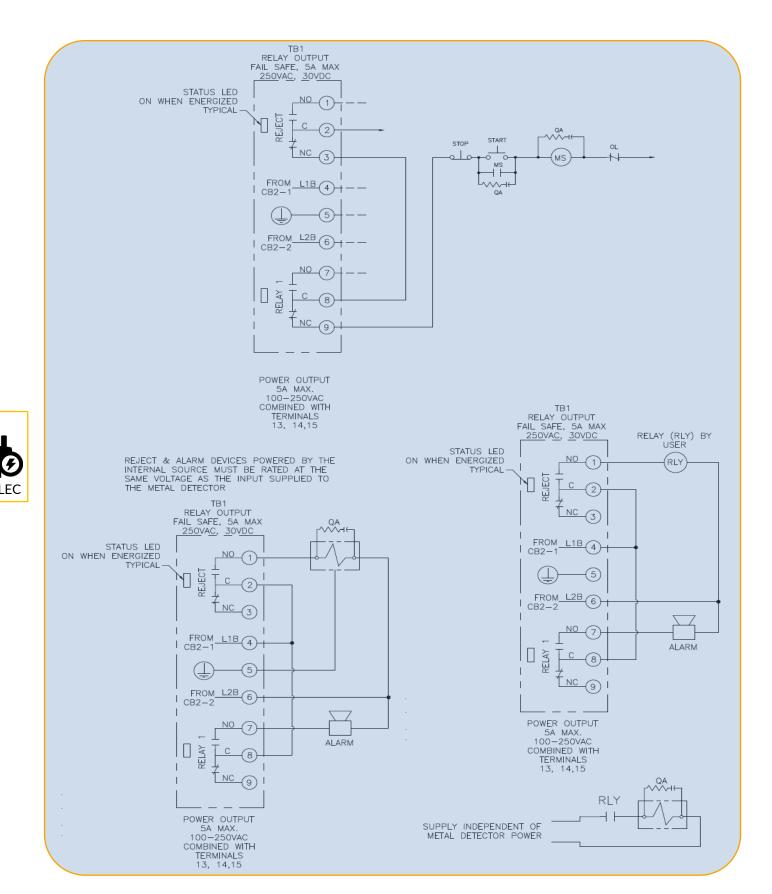
Figure 14: Output connection examples
