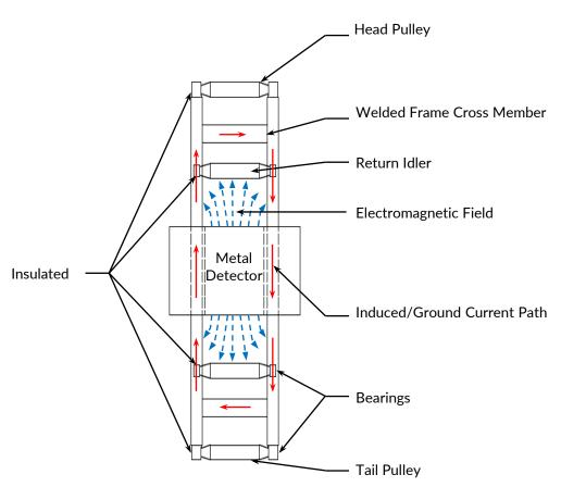
Figure 8: Properly modified conveyor frame for metal detector installation
