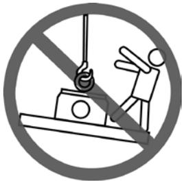
Nobody must be allowed to stand on top of lifted work-piece.
