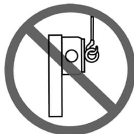
Avoid placing the magnet in shear.
