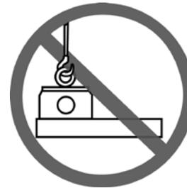
Care should be taken to make certain the load is correctly distributed for the lifting magnet being used.
