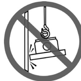
Do not allow load or magnet to come into contact with any obstruction.
