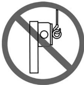
Avoid placing the magnet in shear.
