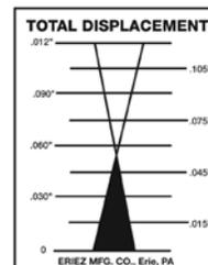
Stroke gauge under vibration (shown at .055" displacement)
