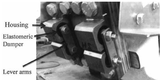
**Figure 11: Elastomeric Damer Components**
