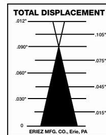
Stroke gauge under vibration (shown at .090" displacement)
