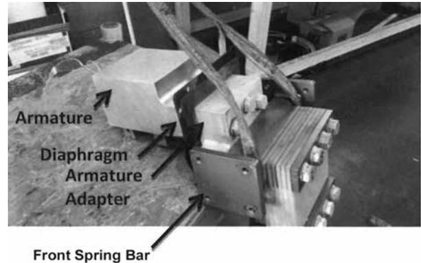
**Figure 14: Armature Removal**
