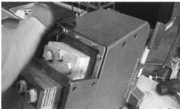
**Figure 12: Diaphragm Removal**
