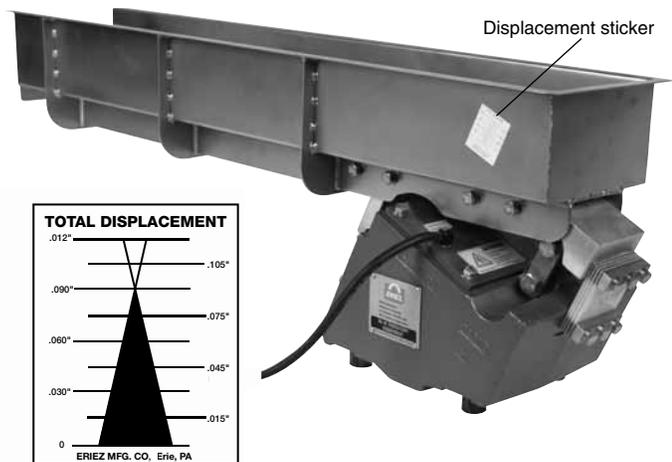
Stroke gauge under vibration (shown at .090" displacement)
