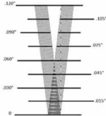
Deflection sticker showing .060" of total deflection. Each unbroken horizontal line above that zero line represents .015" of total deflection. Numerical scale will actually be blurred.
