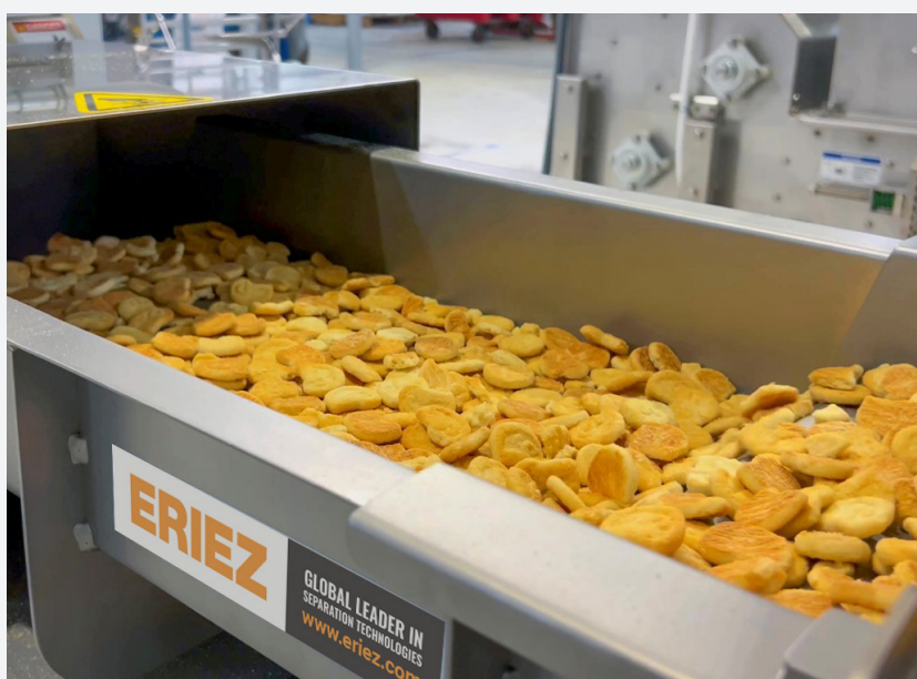
An Eriez Vibratory Feeder metering out product into the X-ray Inspection System
