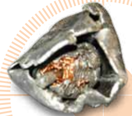
Copper "meatball" from an electric motor
