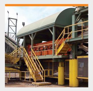
Shred1™ from Eriez uses a combination of magnetics and ballistics to efficiently separate iron-rich ferrous from much of the mixed metals post-drum magnet flow. This new separator delivers two distinct fractions: a premium low-copper ferrous product (in the range of 0.16-0.20% cu) and a traditional #2 shred.
