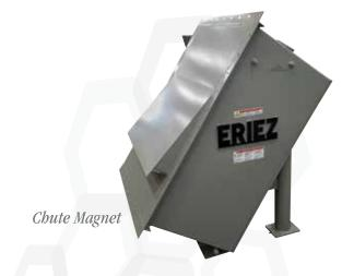
The standard **chute** separator is equipped with support legs designed for installation in a 50° chute as shown, but can be easily modified for greater or lesser slopes as required. An access door built into the chute-work below the magnet is necessary for the periodic removal of accumulated tramp iron. The cooling oil fill and drain connections are readily accessible with the magnet in position.
