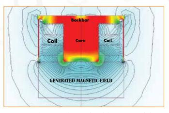
Finite element analysis and modeling a suspended electromagnet's magnetic field.
