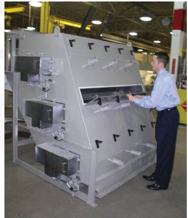
three-roll separator with 6" diameter magnetic rolls
