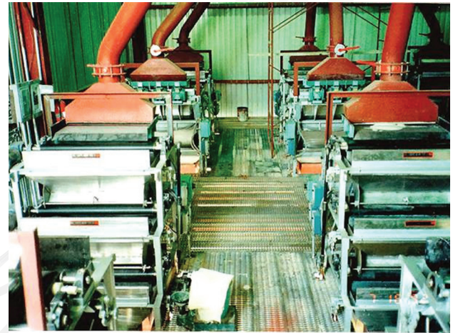
several three-roll separators treating feldspar
