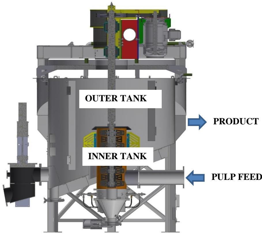
Figure 2. A StackCell cut-away showing the concept of a tank within a tank. The concentric inner tank where particle collection occurs as well as the outer tank, where particle recovery occurs are shown.
