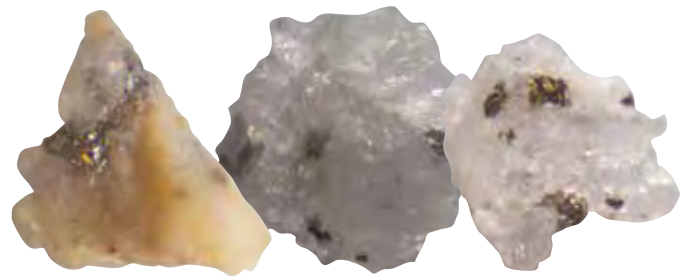
Rejects only those particles that have no hydrophobic surface expression
