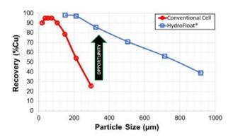
Industrial rougher recovery by size data from a copper concentrator in South America (Conventional vs HydroFloat)
