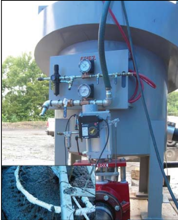
Figure 4 - 1.2-Meter (4-ft.) Pilot Cell with Typical Froth Washed Product (inset).
