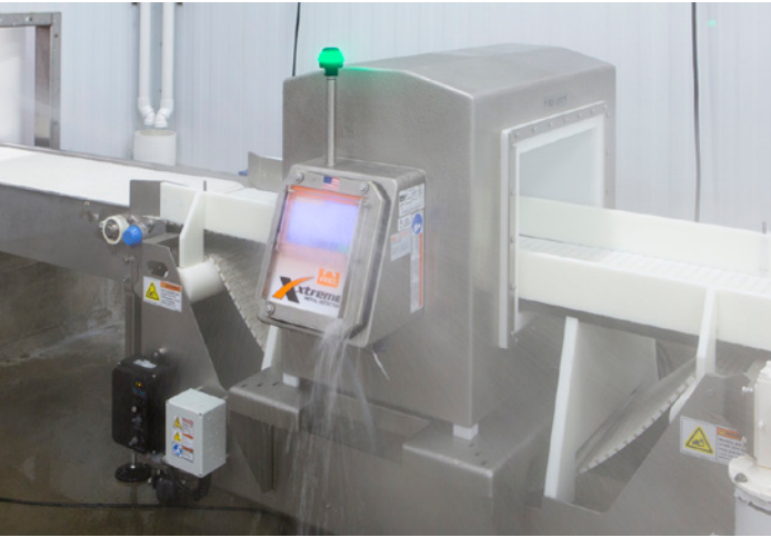
An Eriez Xtreme Metal Detector is positioned at the end of a packaging line that mainly handles Smith's hot dogs and sausages
