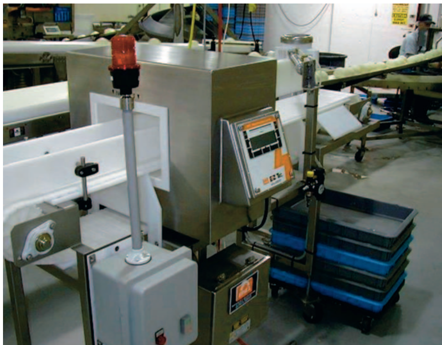
The supplier custom-designed a metal detection and reject system for each of the company's processing lines.
