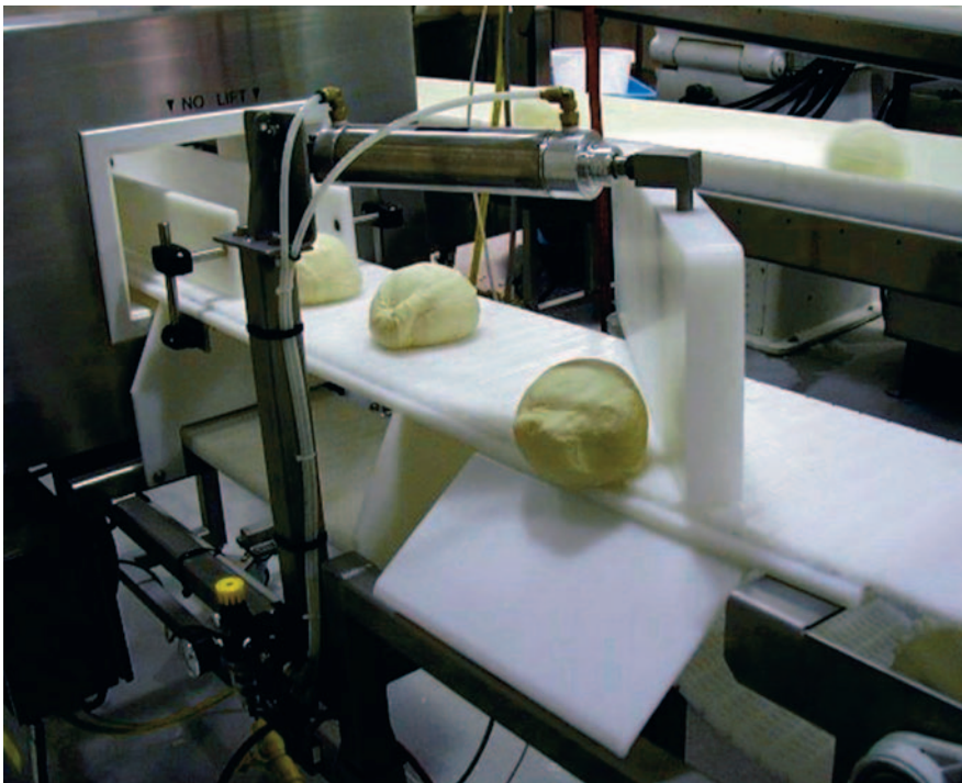
The reject system's diverter arm sweeps across the conveyor's top to remove a contaminated dough ball from the reject zone.
