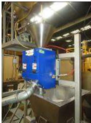
Ez-Tec 9100 inspects plastic granules before the extrusion process, removing any metal contamination.
